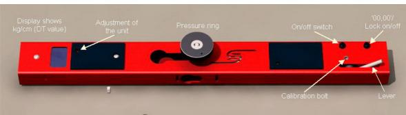
The picture shows the functions of the Stringlab 2 measuring system:
